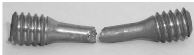
Fig. 7 Fractured sample after tensile test with cup–cone fracture
